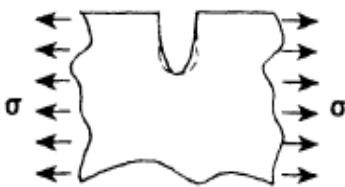
Fig: 3 U-shaped Notch in semi-infinite plate having uniaxial tension
