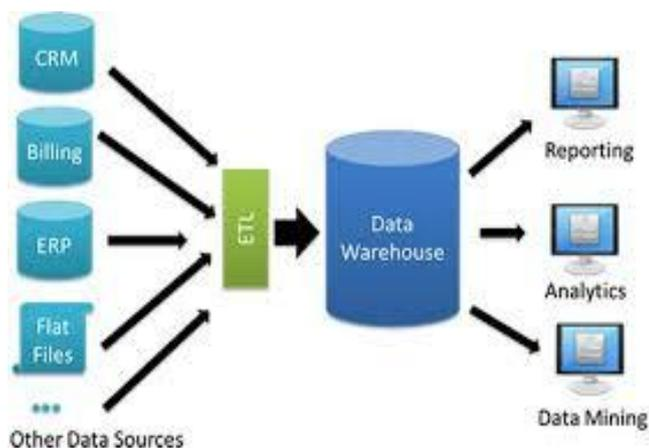
Data Warehouse refers to a database that is maintained separately from an organization’s operational database .A subject oriented, integrated, time variant and non volatile collection of data in support of management decision making process is called as data warehouse.
