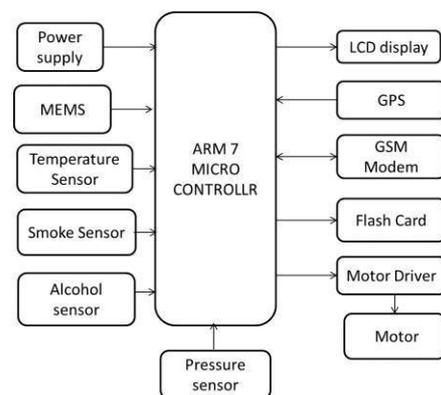
The process of working of this project is explained as follows. the entire equipment of this project is placed inside a vehicle isn't visible to others. Here we have MEMS accelerometer which can sense the movements of the vehicle continuously. When an accident occurs to the vehicle the movement of the vehicle while the incident is happening will be detected by the MEMS and this data is given to microcontroller. Here we use GPS module to track the location of the vehicle where the
