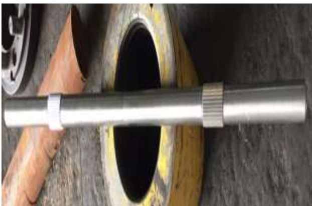
Figure 3.2: Shaft used for our dynamometer
