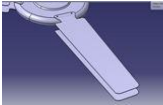
Fig.5; Close look of double plane blade ceiling fan
