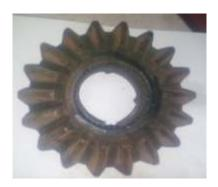
Two important concepts in gearing are pitch surface and pitch angle. The pitch surface of a gear is the imaginary toothless surface that you would have by averaging out the peaks and valleys of the individual teeth.
