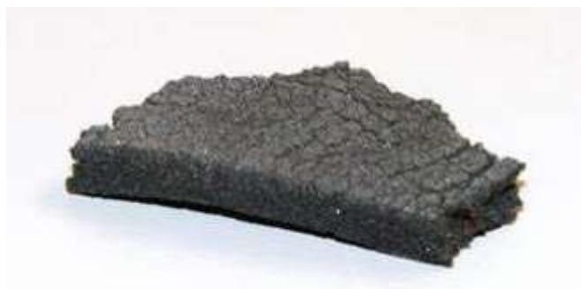
Fig. 2- Abrasion in rubber product[18 ]
