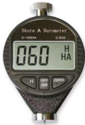
Fig. 5- Durometer to measure hardness[20]
