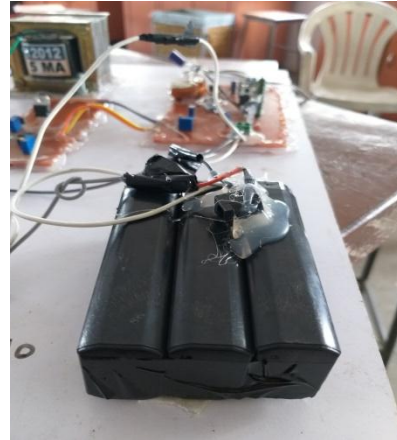
Fig: 3.8- 4V Battery pack
