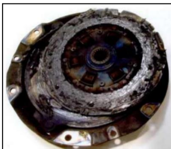
Fig. 1- Friction Material affected by Heat [2]
