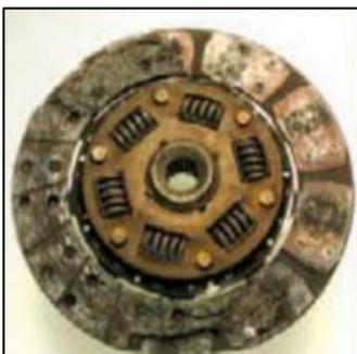
Fig. 2- Fault due to clutch slip [2]
