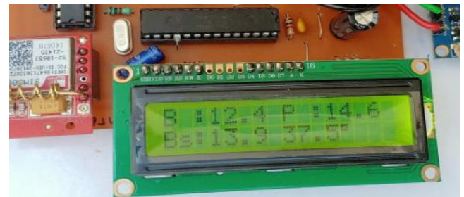
Fig.-5. a) Showing solar panel output with engine temperature
