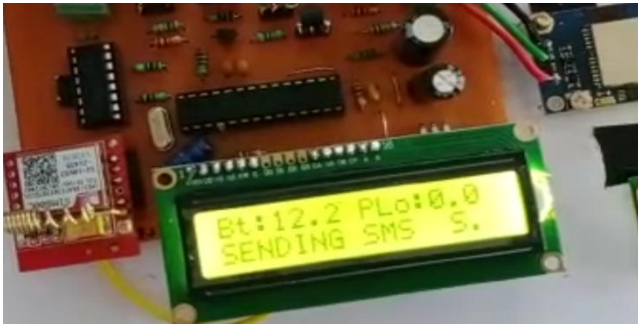
Fig.-5. e) Sending message and location when vehicle stolen
