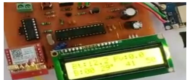
Fig.-5.b) Displays vibration sensor output when vehicle tilted (in case of accident)
