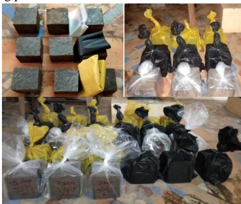
Fig.-7 Concrete cube are cover by 3 different colour polythene for curing
