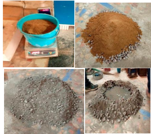
Fig.-2 Weight batching and mix of concrete
