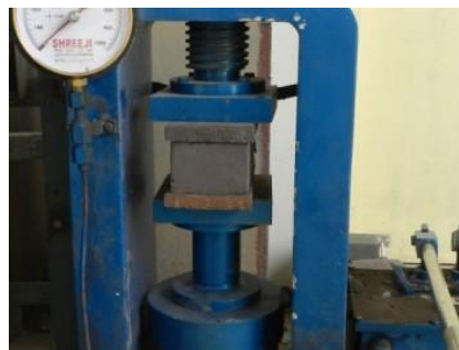
Figure-8 Testing of cubes for compressive strength
