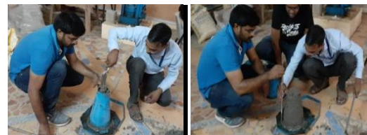
Fig.-3 Slump test of concrete
