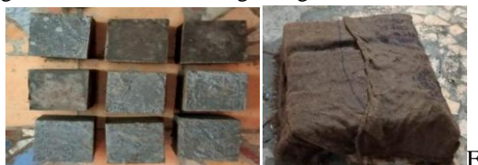
Fig.-6 Concrete cube are cure by wet jute bag for 30 minutes before cover by polythene
