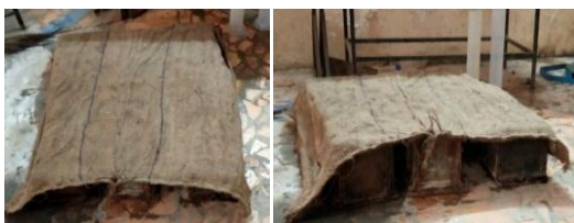
Fig.-5 Concrete cube cover by wet jute bag for retard moisture loss
